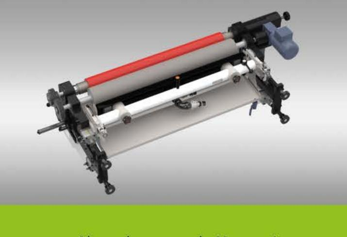
Dr. Chamber Bıçak Sistemi ve Seramik Aniloks (Std.) Dr. Chamber Blade and Ceramic Anilox
